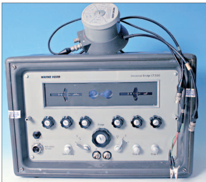
● Fig. 3: A Wayne Kerr Universal Capacitance/Inductance Bridge. This American made unit is extremely useful, and should always be purchased (if possible) with the remote low capacitance/inductance head (low impedance adapter) on top of the cabinet. This model cost G3XFD £14 at a QRP rally (see text).
