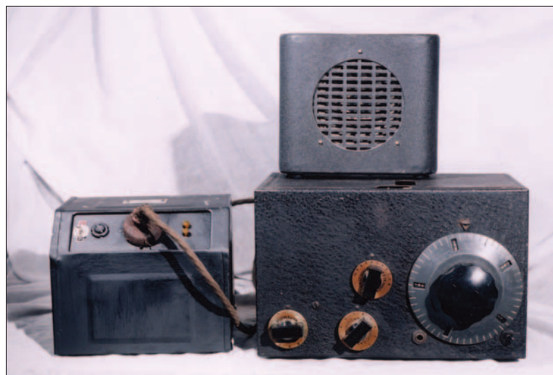
● Fig. 1: The HRO 1-10 v.h.f. receiver with power supply and speaker. The aerial connects through hole in lid of set (see text).
