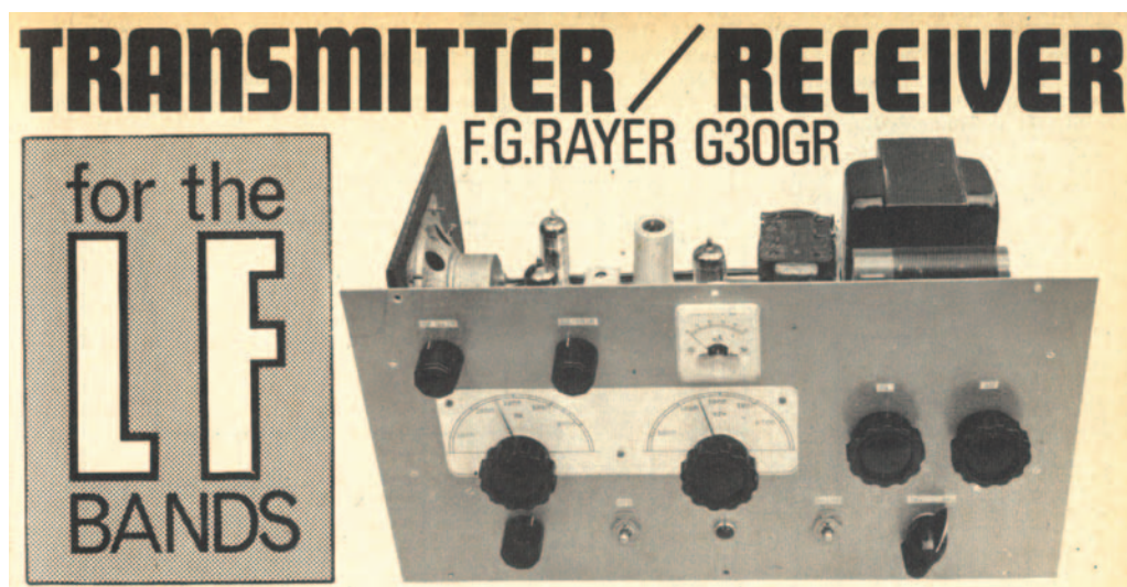
● The prototype G30GR 1.8/3.5MHz a.m. transmitter-receiver. This project is still viable says G3XFD and he suggests you'll find much of what you'll need in your junk box!
