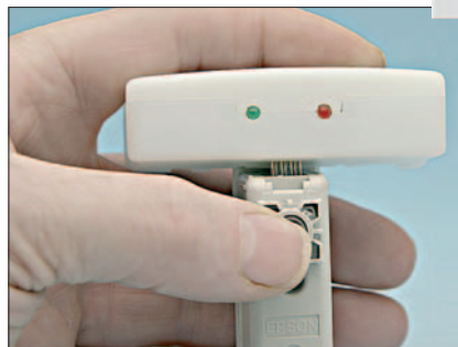
● Fig. 3: In use the device is pressed against the pins of the chip. See text for more details.
