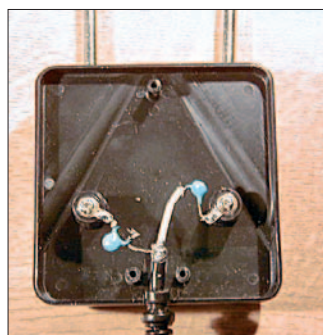
● Fig 1: Inside the original unit are the two series safety capacitors (blue) these are removed (see text).
