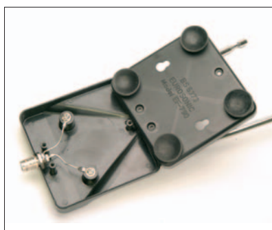
● Fig. 3: After fitting the BNC socket and wiring the elements in. Note the four 'suckers' that provide a good grip on window glass.
