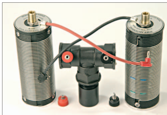
● Fig. 3: The antenna comprises of two 0.558m long (22in) anodised aluminium elements, two well constructed loading coils (shown here), and a pair of stainless steel telescopic whips. The assembled legs attach to the 'T' piece (centre).
