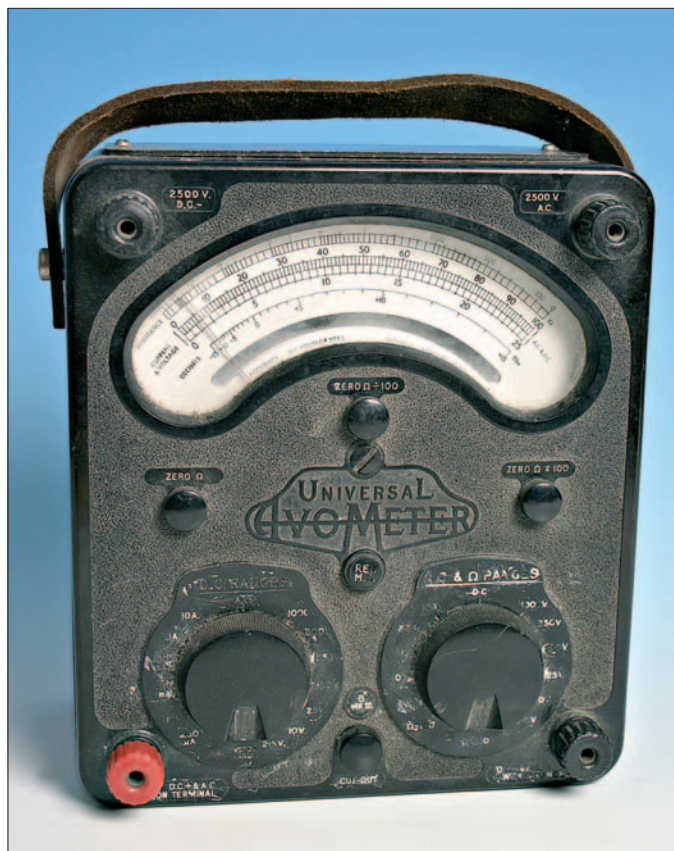
● Fig. 1: The AVO multimeter - very old nowadays perhaps - but incredibly rugged and with many superb features. This Model 8 Mark III cost £1 at the Leicester Amateur Radio Show, and the only problems it had (the loss of white lettering-infill in the engraved markings, as can be seen from the photograph) is easily overcome. The most expensive item G3XFD had to buy for the meter was a specialised battery which cost £2 (see text).
