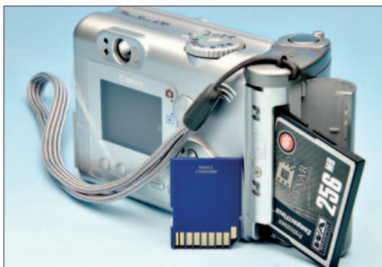
Fig. 8: A Canon A70 digital camera with a 256MB compact flash memory card. The smaller blue card is an Secure Data (SD) type from another camera. As with other cameras, using the rear-mounted screen, drains battery power quite quickly.
